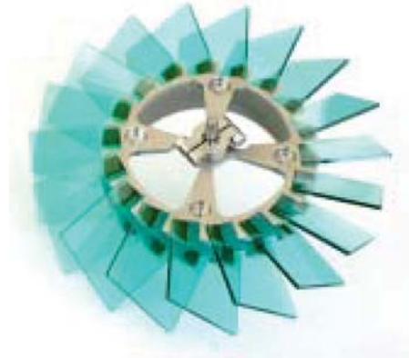
Figure 1: Picture of the wheel of the rotating light trap.
